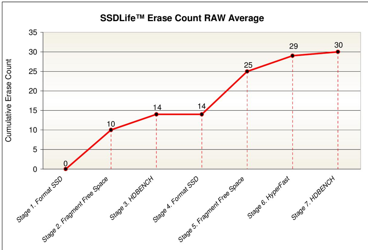
Figure 7: Cumulative Erase activity on 8GB PATA SSD as measured by SSDlife software.
