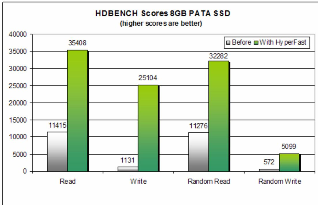
Figure 4: Benchmark scores on 8GB PATA SSD with HDBench software.
