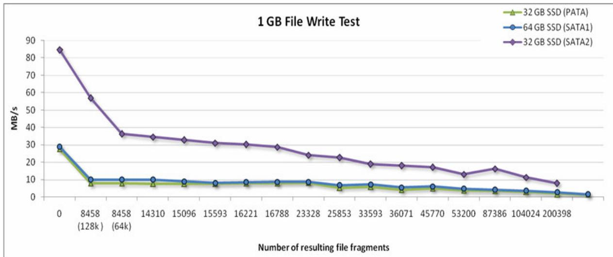
Figure 2: Write I/O throughput degradation due to fragmented free space.
