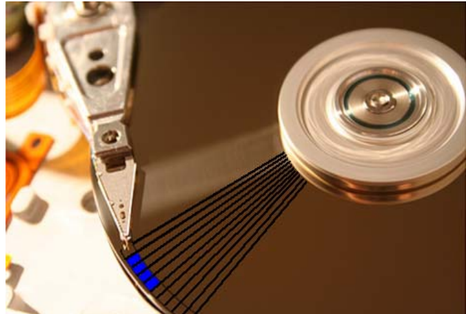
Figure1 – Sectors on a disk formed into a 2KB cluster
